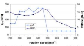
Fig. 6. Optimal air overpressure  $p_{pS}$  and RMS  $M_k$  value in relation to the rotation speed of mechanical system
