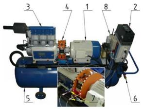
Fig. 2. Implemented torsional oscillating mechanical system
